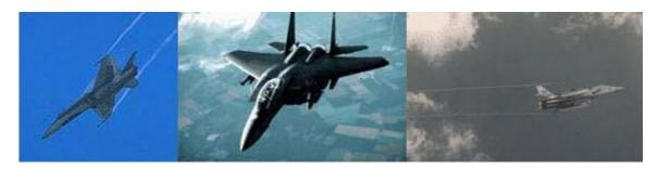
A different type of contrail or condensation trail is caused when a wing surface or winglet causes a cavitation of air in very humid conditions. This results in a unique vapor trail that is not formed due to exhaust gases. The next time you fly in a commercial aircraft through a rain cloud, look for the vapor trails that form over and around the wing. Typical fighter wingtip contrails are shown below.
