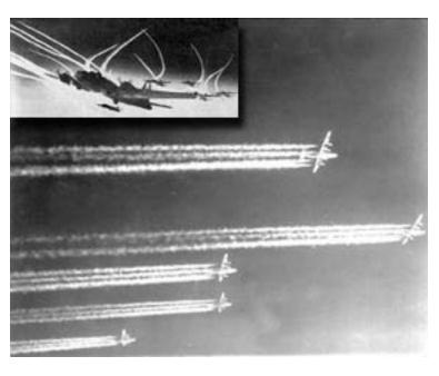
evaporate quickly or they can persist and grow. Engine exhaust produces only a small portion of the water that forms ice in persistent contrails. Persistent contrails are mainly composed of water naturally present along the aircraft flight path.
